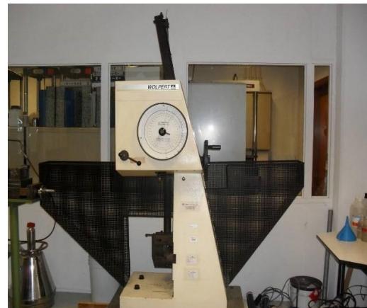
Figure 11 - Examples of impact test pendulums; a) modern computerised equipment, fully enclosed for safety; b) older manual equipment with only partial protection.
