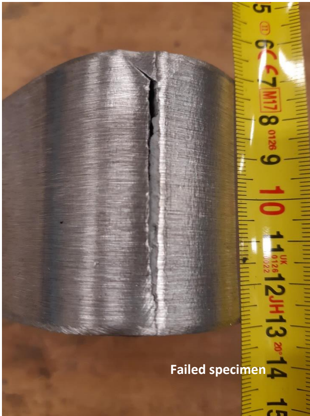
Figure 49 - Images of acceptable result (no imperfections after the test, see top image) and not acceptable result (failed specimen: bottom image) according to ISO 15614-1.
