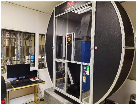
Figure 11 - Examples of impact test pendulums; a) modern computerised equipment, fully enclosed for safety; b) older manual equipment with only partial protection.
